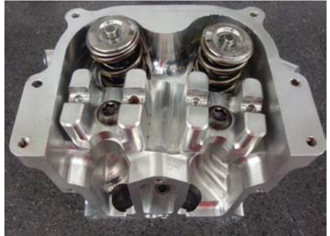
Billet aluminum cylinder heads with dual plugs.
