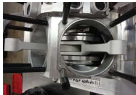
Billet aluminum connecting rods that made in house @ S&S shown along with the beefed up redesigned case made from billet aluminum as well.
