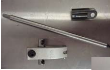
Rocker arm, pushrod and lifter used in the Pro Stock Motorcycle V-Twin engines.
