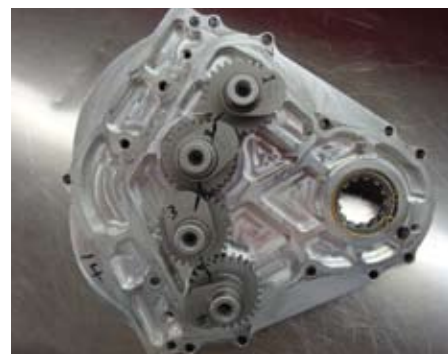
Four individual camshafts shown installed in the billet aluminum case.
