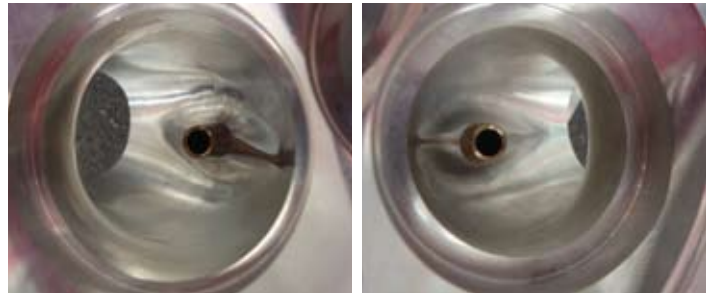
Picture above left is the intake valve seat and intake runner. Picture above right is the exhaust valve seat and exhaust port on the billet aluminum cylinder heads.
