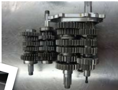
Suzuki 6 speed transmission that is put in the V-Twin case.
