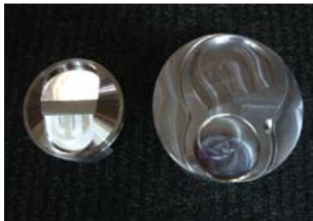
Comparing the 5 1/8" piston used in this engine to a standard size bore piston.
